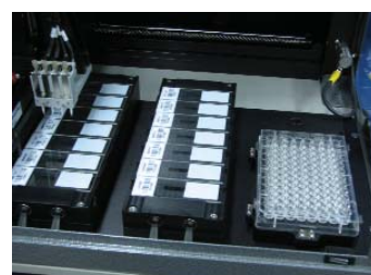
Close Up photo of an AD1500 configured with a 14 glass slide nest
