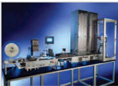
Figure 3. A reel-to-reel system by BioDot Inc. (Irvine, CA) with camera control and dry towers.
