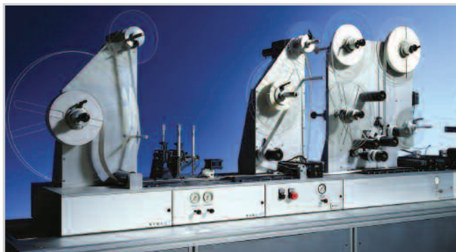
Figure 2. An auto-laminator system by BioDot Inc. with backing card feeding module, dispensing module, and laminating module.
