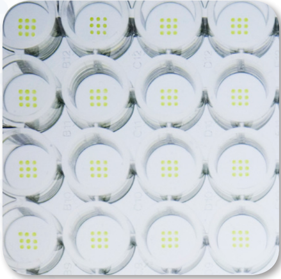
3 x 3 array dispensed into a 96-well microtiter plate.
