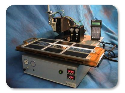
The AD3200 is a workstation designed for development and pilot scale production. Its standard 8 BioJet Plus and nine-plate nest configuration makes it ideal for a medium throughput Biosensor laboratory.
