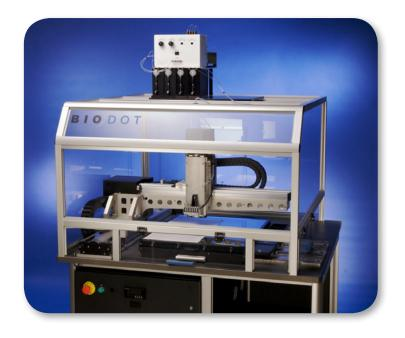
The AD6000 is a workstation designed for high throughput biochip manufacturing. Vision inspection (CCD camera) and barcode reading can be configured on the AD6000 for verification of substrate positioning and reagent spot dispensing.
