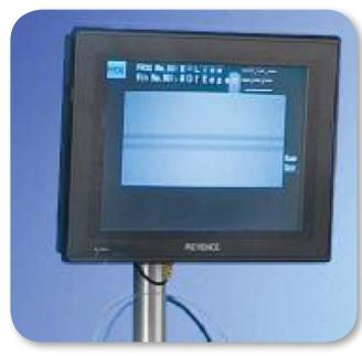
The BioDot VS1000 Inspection Vision System is designed to perform automated line inspection and marking for lateral flow test manufacturing. The system can be integrated onto any of BioDot's XYZ or Reel-to-Reel products (hand-held terminal controlled).
