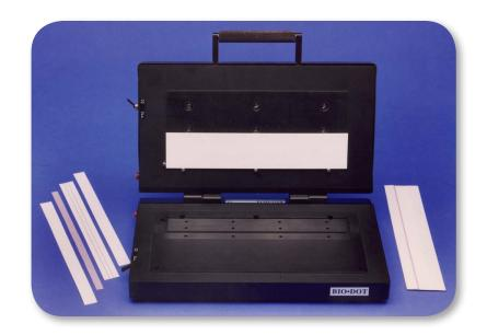
The LM5000, also known as the Clamshell, is a manualluy operated module designed for the accurate assembly of precut materials into a specific test strip product. Precut membrane, absorbent material, conjugate pads and plastic backing are brought together to form a laminated lateral flow test strips. The Clamshell Laminator offers maximum productivity for a manually operated system.
