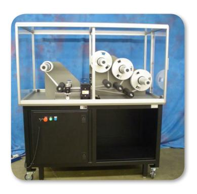
The Rotary Slitter is a high-speed precision slitting instrument used to slit web materials up to 300 mm in width into thin webs down to 5 mm in width. The minimum cut width will be application limited. The slit webs are collected in roll formats on take-up reels. The slitting process is enclosed in a cabinet with safety interlocks.
