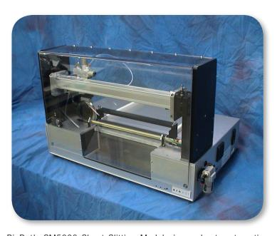
BioDot's SM5000 Sheet Slitting Module is a robust, automatic slitting system used to cut sheet material into smaller widths. Cut width, cut speed and number of cuts are easily programmed through BioDot's handheld terminal. Programs may be saved for future reference. The SM5000 is equipped with a set of variable guides for the accurate in-feed of the sheet material. A position sensor senses the sheet edge for correct cut positioning and precise slitting.
