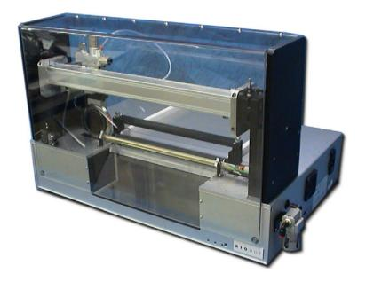
BioDot's SM5000 Sheet Slitting Module is a robust, automatic slitting system used to cut sheet material into smaller widths. Cut width, cut speed and number of cuts are easily programmed through BioDot's handheld terminal. Programs may be saved for future reference. The SM5000 is equipped with a set of variable guides for the accurate in-feed of the sheet material. A position sensor senses the sheet edge for correct cut positioning and precise slitting.
