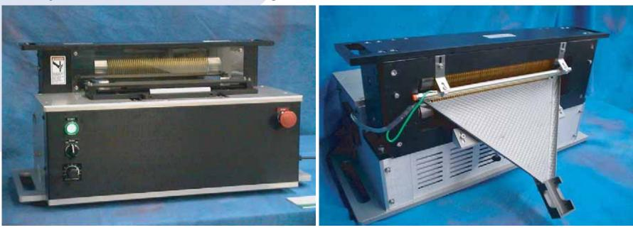
The equipment package also includes an Inline Rotary Slitter for conversion of wider webs to narrower webs for the lamination process.
